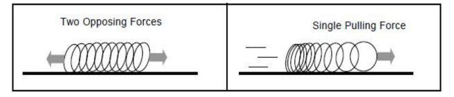
However, with only a **single** continual pulling force on **one end**, shown on the right, the coils stretch more at the *leading* end as they strain to continually accelerate the ongoing resisting inertia of the rest of the spring. In this case, there is successively *less* stretch toward the *trailing* end as there is successively less trailing-coil mass to cause inertial drag.
